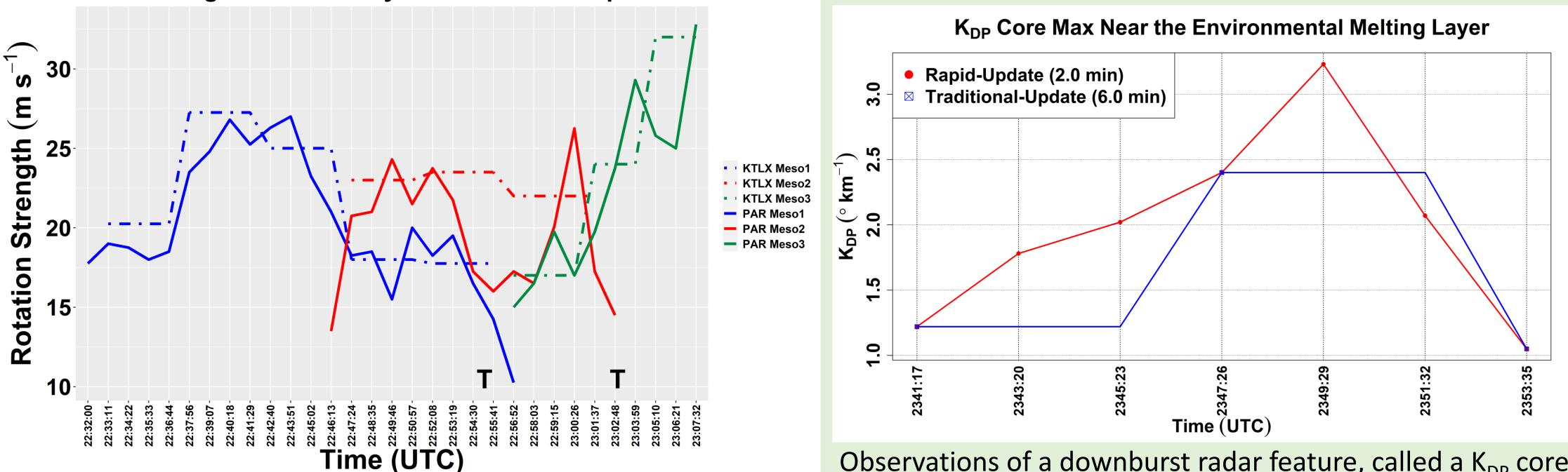
Observations of rotation in a supercell by a PAR (solid lines) and radar in the current radar network called KTLX (dashed lines). T marks the time of tornado formation.
